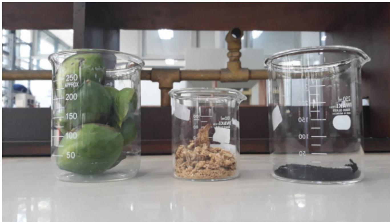
Three UGM students have researched the use of country almond (*Terminalia catappa*) waste into activated carbon for cobalt-molybdenum bimetallic catalyst in plastic waste hydrocracking process.
