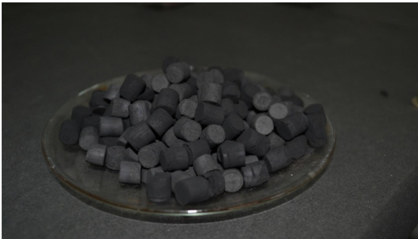
YOGYAKARTA - A lecturer in Chemical Engineering of UGM, Ir. Imam Prasetyo, M.Eng., Ph.D., has developed a technology in storing gas using cartridge, done by gas adsorption through porous carbon. This is expected to solve the problem of energy conversion from fuel to gas. There are concerns among people in using gas due to possibilities of gas explosion and the expensive cost of gas compression.
